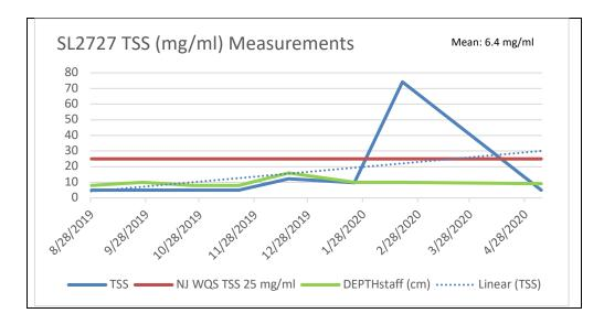
Link to online continuous sensor. Data collected on conductivity, water temperature, and depth. Note while values for turbidity are listed, the sensor is not set up for taking turbidity readings due to the shallow nature of the stream:
