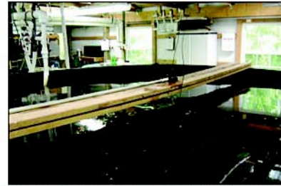
Boom over tank, from which remote camera is suspended
